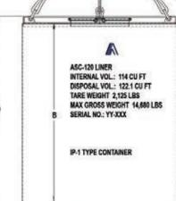
Example: ASC-120-G-PDX is a 120-ft<sup>3</sup> steel container with grapple top and powdex internals.
