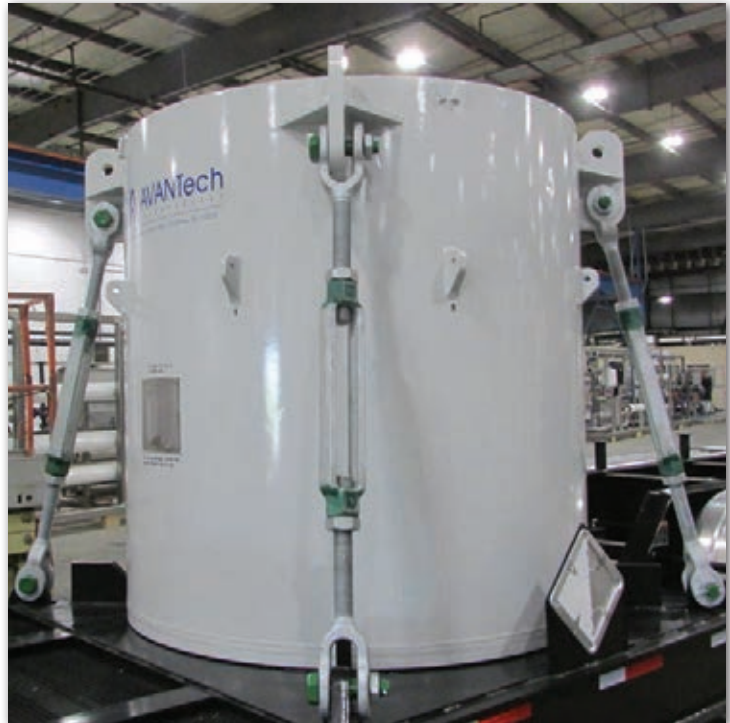
ATS-215 Shipping Cask on Transport Trailer
