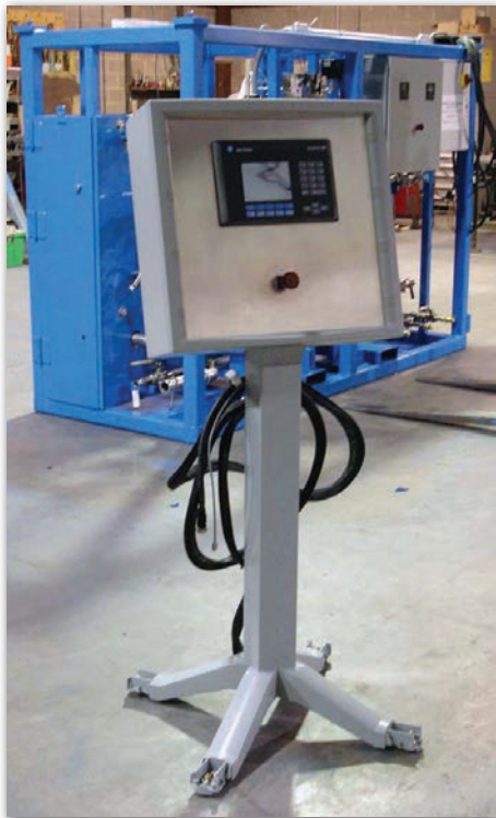
Stand-alone pedestal with Programmable Logic Control (PLC) touch screen controls permits easy, remote operation.
