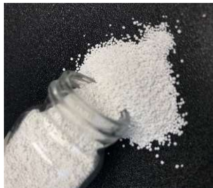
Fig. 7. Crystalline Silicotitanate Media
