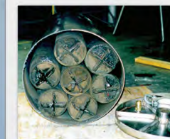
Filter Membranes in SCF™ Canister (top of canister has been cut off for viewing). Note high dirt loading on depleted filters.
